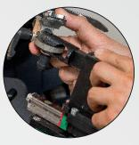
The holder allows you to control the quality of the tool's sharpening while maintaining its position.
